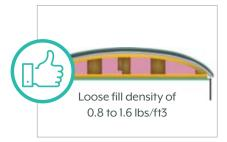
FULLY INSULATED BOWED ROOF TO CONSISTENT DENSITY
